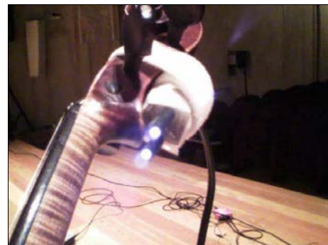
Figure 2. MicroLED for the encoding of the parameter distance of the left hand from the sensor.
